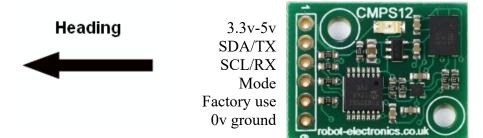
For **I2C** the mode pin can be left open or pulled to the supply voltage, for **serial mode** the mode pin should be connected to 0v ground.
